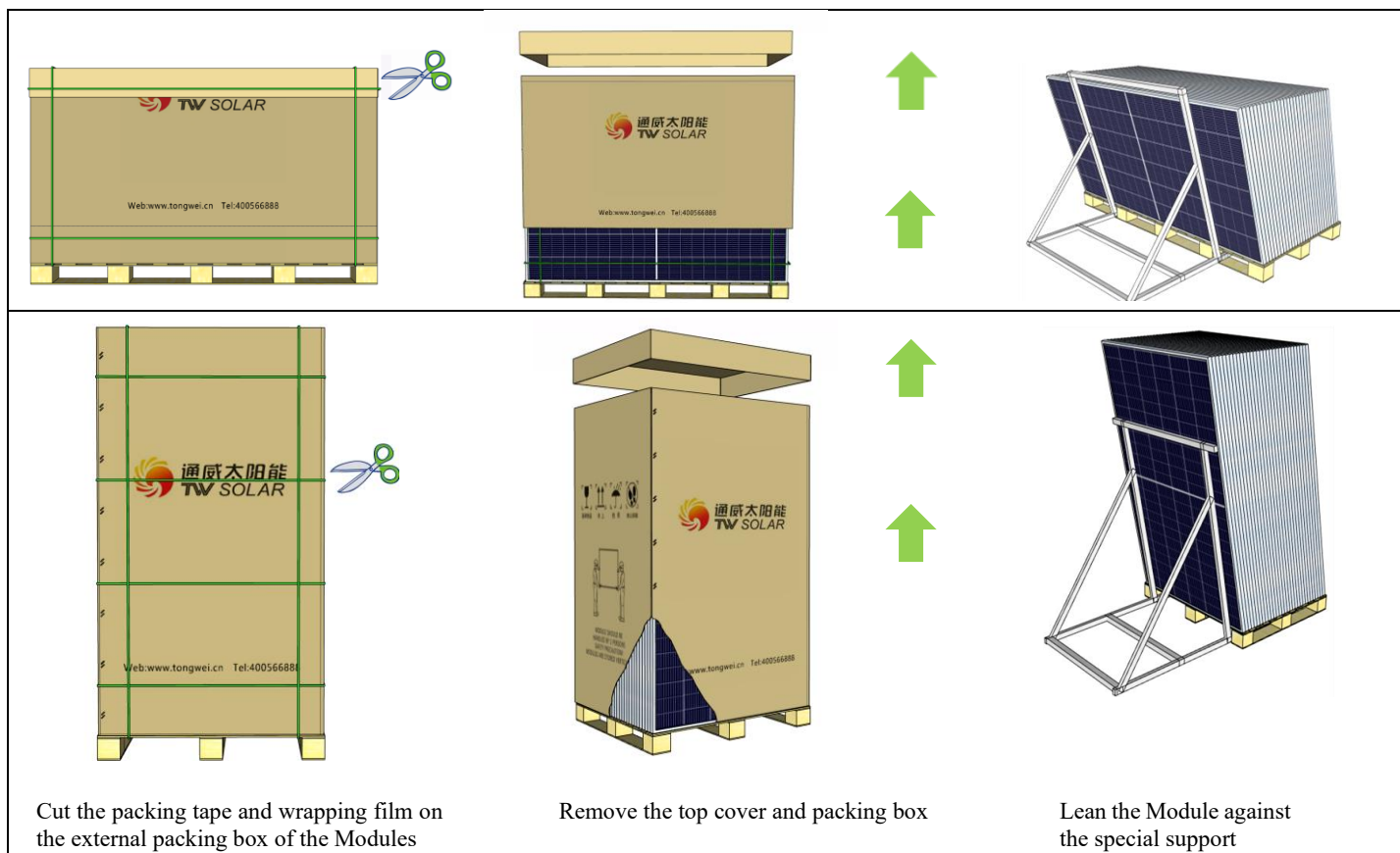
Figure 13 Schematic diagram of the unpacking procedure of the Module
